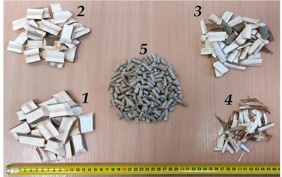
Figure 2. Fractional composition of the fuel from the biomass of a fast-growing willow Salix Viminalis : 1 – a large fraction, 2 – a medium fraction, 3 – a small fraction, 4 – a very small fraction, 5 – fuel pellets
