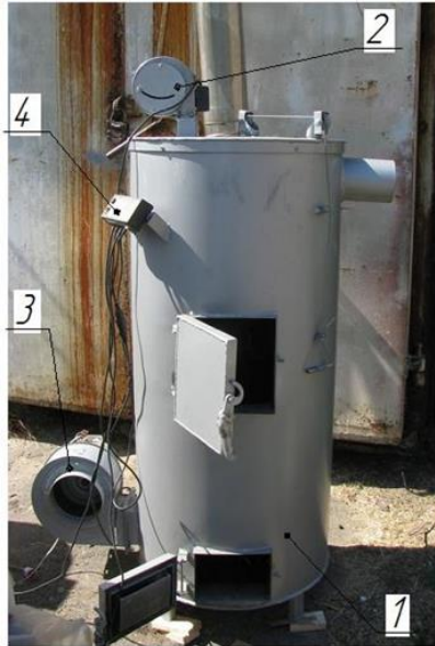
1 – boiler, 2 – fan WPA-06, 3 – fan OBR-200M-2K, 4 – electronic control system ATOS, 5 – fuel, 6 – air supply system
